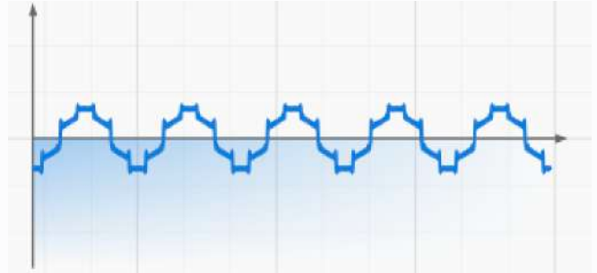
IEC61000-4-13 Odd harmonics that are not multiples of 3 @Class3/50Hz
